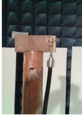
Figure. 11. Designed antenna into anechoic chamber.
